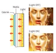
Single-layer printing looks faded when the illumination is on because too much light is transmitted.
